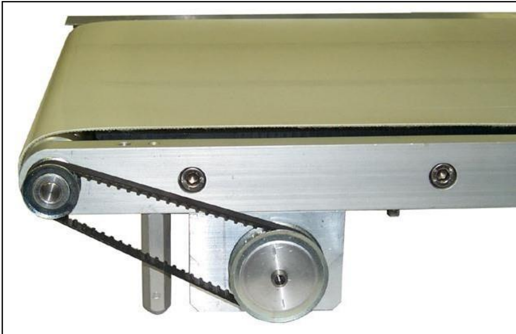
Figure 7- 5 - Section of the conveyor belt with motor
