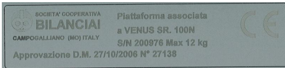
Figure 1- 9 – Metrological data plate - M.D. type approval
